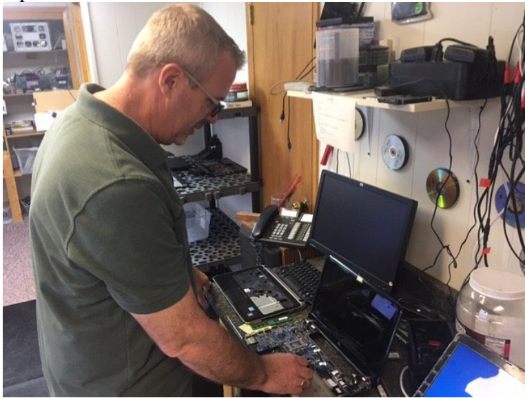
Figure 4: Steven examining a damaged motherboard in a laptop computer that is going to be replaced.
