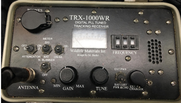
Figure 3. Tracking receiver with frequency gages and cable hook-up for the antenna.
